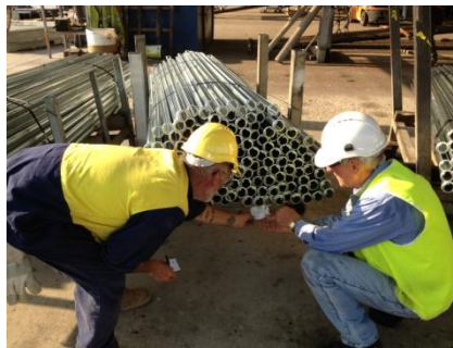
QA Inspection & Tag Recording
