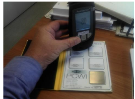
Calibrating Thickness Tester
