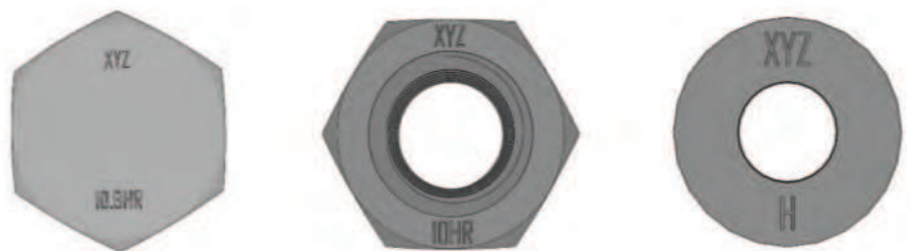
Figure 12: Marking for class 10.9 High strength bolts, nuts and washers
