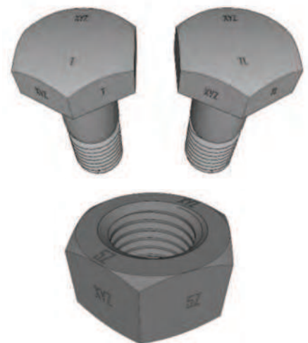
Figure 9: Marking For Tower Bolts And Nuts
