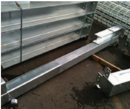
Figure 9 While not a welding defect, steels of different compositions that have been welded together in the same plane prior to galvanizing can result in a differing appearance after hot dip galvanizing
