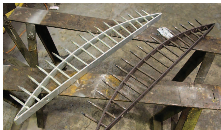
Figure 13 Restoration for Sydney Water of an old spike guard was successfully completed using GMA braze welding
