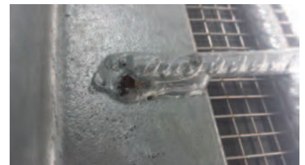
Figure 2 A porous weld has allowed pre-treatment solutions to become trapped inside, resulting in a bare spot near the weld
