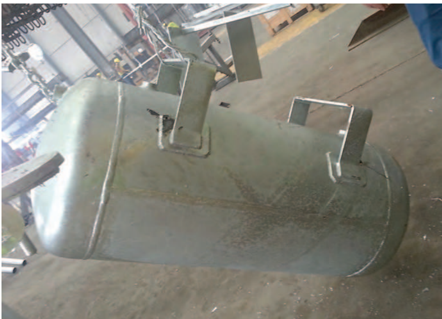
Figure 8 Blowout from undersized hole for venting the overlapping area of the plate fully welded to the large hollow vessel
