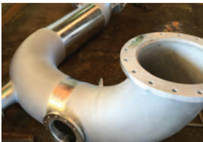
Figure 10 Another example of steels of widely different chemical composition causing an initial appearance issue for the customer. In most cases this affect is aesthetic and there is usually no detrimental effect to the durability of the article
