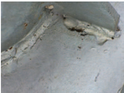
Figure 1 Poor welding practice can lead to areas of uncoated steel and result in surface conditions that collect moisture and detritus both leading to a reduced service life
