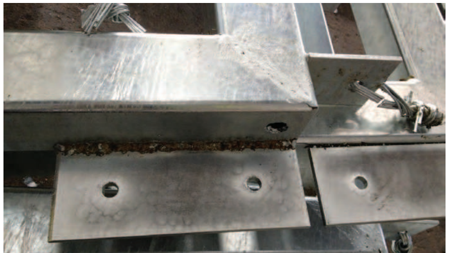
Figure 7a Welding slag hasn't been cleaned by the fabricator after welding and has created a bare spot
