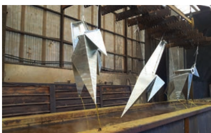
Figure 6: The complex sculptural shapes in “The Moment” meant that only a hot dip galvanized base with an aesthetic top coat would meet to the requirements of the sculptor, Damian Vick.
